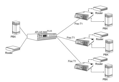
Figure 1-1. Point-to-Point Circuit
